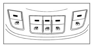
The window switches for all doors are located on the center console. A window switch for each rear window is located on each rear door.
