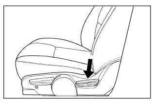
Driver's Seat with Manual Recline and Manual Height Adjuster shown
