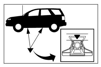
6. Find the arrow on the plastic lower body panel. Position the jack head under the metal jacking flange and not the plastic lower body panel.
