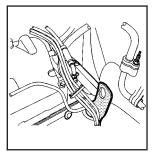
The remote negative (–) terminal is located in the front of the engine compartment, near the engine oil dipstick.
