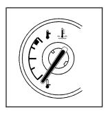
This gage measures the temperature of the vehicle's engine.
