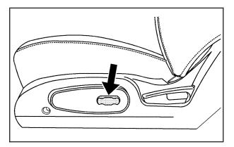
If the vehicle has a power seat, the control used to operate it is located on the outboard side of the driver's seat. To adjust the seat do any of the following:
