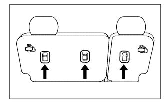
The top tether anchors for each rear seating position are located on the back of the rear seatback. You may need to adjust the rear compartment storage panel/cover in the rear cargo area to access the anchors. Be sure to use an anchor located on the same side of the vehicle as the seating position where the child restraint will be placed.
