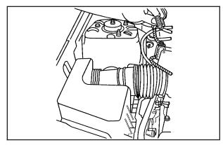
Disconnect the air flow sensor electrical connector.
