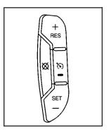
The cruise control buttons are located on the left side of the steering wheel.
