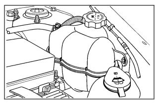
The surge tank is located on the driver's side of the engine compartment. See *Engine Compartment Overview on page 348* for more information on location.
