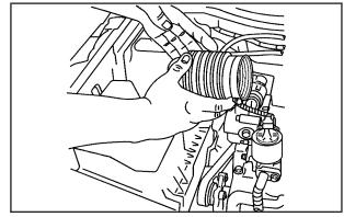
5. Remove the air outlet duct.
