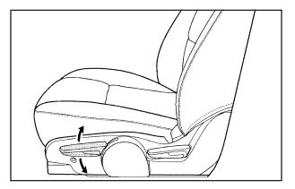
If your vehicle has a manual driver seat height adjuster, it is located on the outboard side of the seat near the front of the seat cushion.
