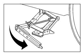
14. Lower the vehicle by turning the jack handle counterclockwise.
