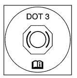
Your brake master cylinder reservoir is filled with DOT-3 brake fluid. See Engine Compartment Overview on page 348 for the location of the reservoir.
