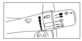
Use the lever on the right side of the steering column to operate the windshield wipers.
