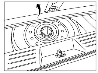
1. Lift the load floor up and pull it out of the vehicle and set it aside.
