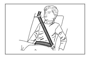
Buckle, position, and release the safety belt as described in Rear Seat Passengers on page 36. Make sure that the shoulder belt crosses the shoulder.
