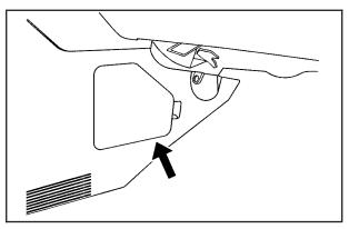
Remove the console cover to access the fuse block.
