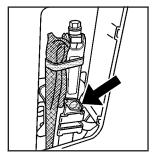
Remove the wing-bolt holding the jack and then remove it.
