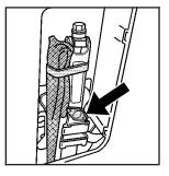
Install the jack in the left side panel of cargo area and secure it with the wing bolt.
